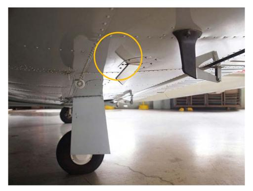
Figure 4. AOA probe on Piper Arrow aircraft
