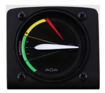
Another common way to communicate AOA to the pilot is using symbols, as shown in figure 5. This type of AOA indicator is often referred to as an AOA indexer.
