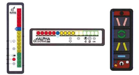
Figure 2. The three AOA indictors preselected by the flight department for the proposed study. vertical bar, horizontal, bar, and legacy indicators.
