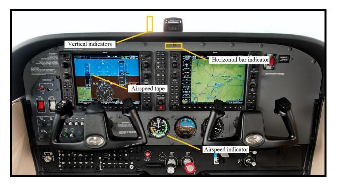
*Figure 5.* Location of the AOA indicators in relation to the airspeed tape on the G1000 and standalone airspeed indicator.
